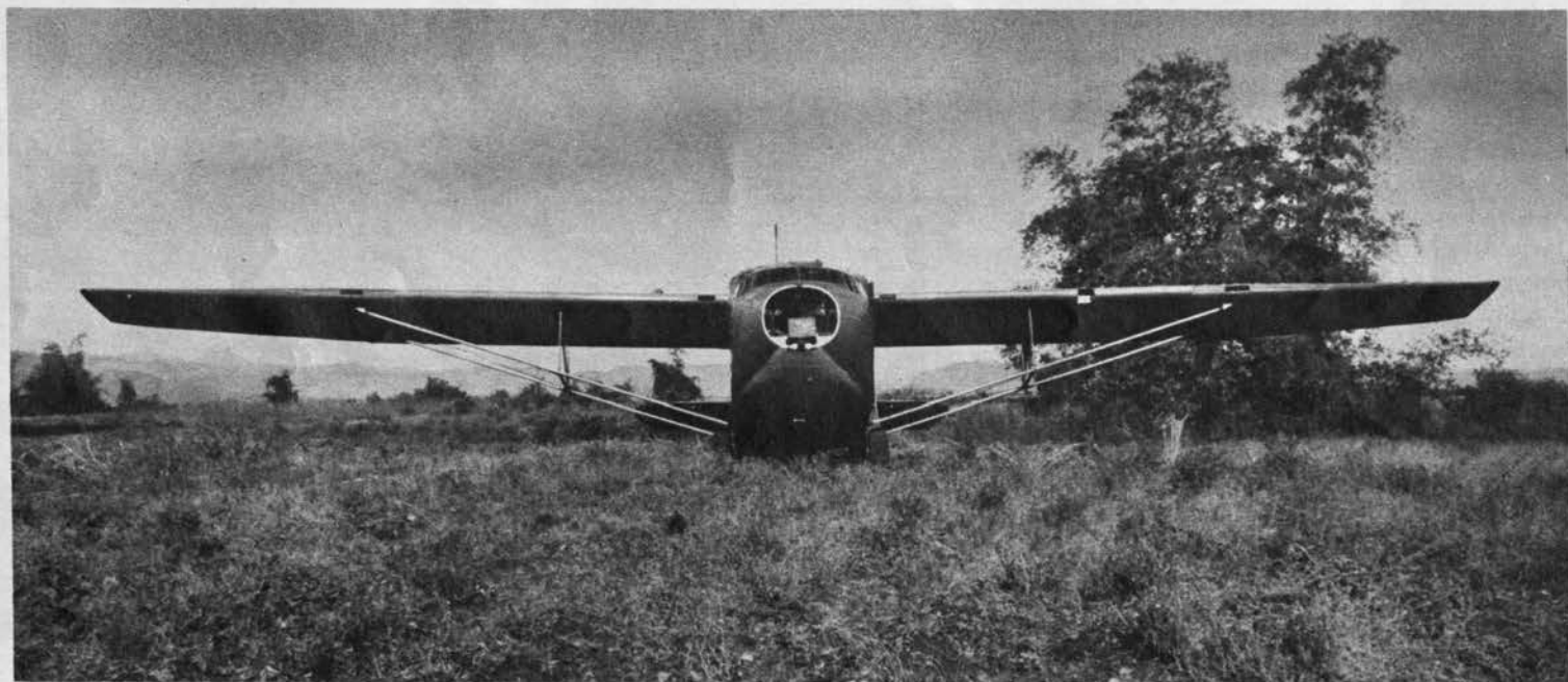
Head-on, the KU-8 shows typical glider features—bulky fuselage and high, broad wing. KU-8 is the first Japanese glider designed to
